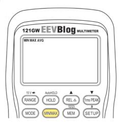
To find the minimum and maximum value found during sampling you can use the MIN/MAX button.
