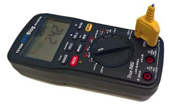
When measuring temperature be sure to have the leads connected as above and in the correct range.
