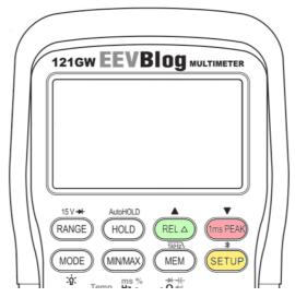
To configure and read settings for the multimeter you can press the *SETUP* button to view the settings. If you press the setup button multiple times you will cycle through the menu, the order of the menu is as follows:
