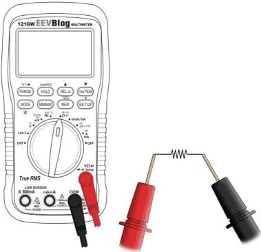
When taking measurements, you must connect the leads as shown above.
