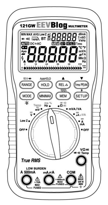
**Digital Display:** Readings are displayed on dual 4  $\frac{4}{5}$  -digit 50,000 count LCD display. One Primary and one smaller secondary function display. The secondary function display is only used when a function that requires it is selected. A fast updating bargraph is below the main display.
